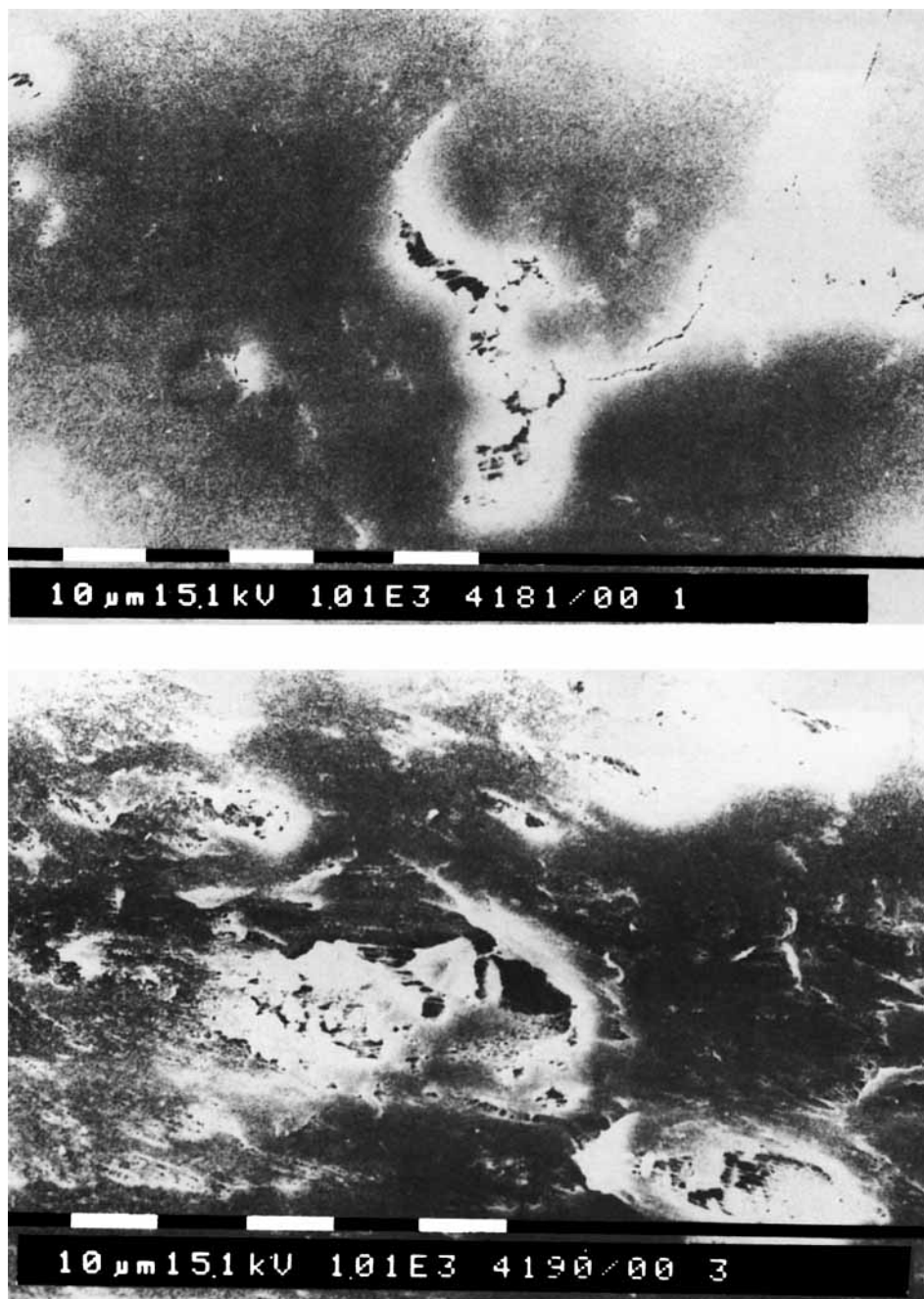
Figure 4 Scanning electron micrographs of the films deformed under the following conditions: l_0 = 1.0 mm, T = 90^\circ\text{C} , w = 20 cm/min, \epsilon is (a) 0%, (b) 100%, (c) 200%, (d) 450%.
